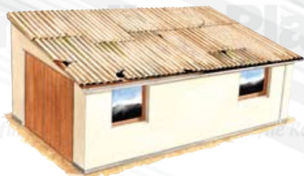
A TYPICAL LEAKING ASBESTOS ROOF
