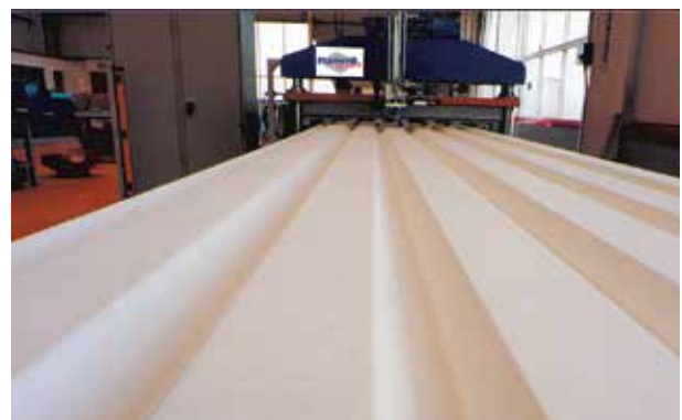
Inside the Planwell factory, manufacturing Permaroof Metal Roof Sheetting
