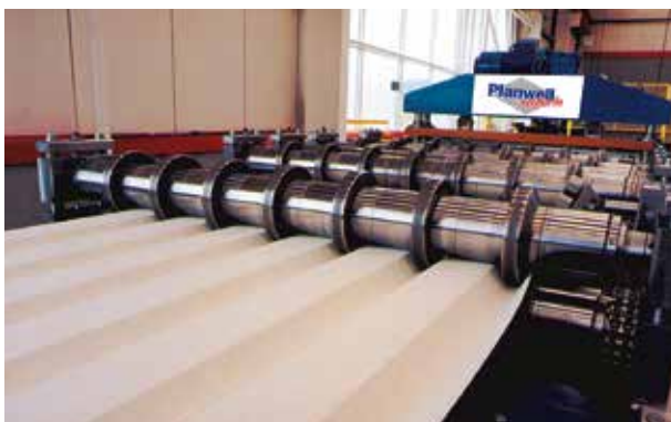
Inside the Planwell factory, manufacturing Permaroof Metal Roof Sheetting
